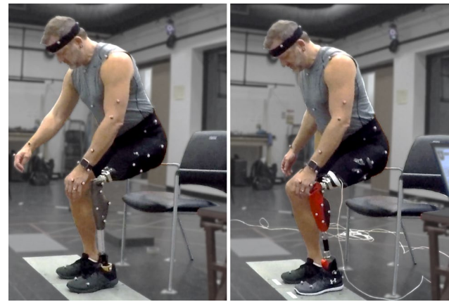
Fig. 1 A subject sitting down with passive (left) and powered (right) prostheses during the experiment. Retroreflective markers on the subject track the movement of their body segments, and separate six-axis force plates record ground reaction forces from each leg. A wire connected to the powered leg synchronized data recording
