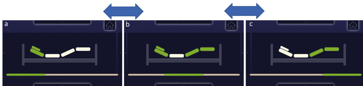
Fig. 6 Control and selection of three position segments from the left: a headrest, b headrest and leg rest, and c leg rest
