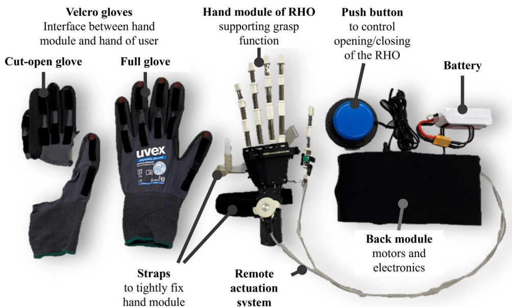
Fig. 1 Overview of the RELab tenoexo RHO system: The fully wearable and portable RHO supports grasp function in people with sensorimotor hand impairment. The hand module is actuated via a remote actuation system. Battery, motors, and electronics are placed in the back module. A full or cut-open glove and straps allow to fix the hand module on a user's hand. A push button is used to trigger opening/closing of the RELab tenoexo
